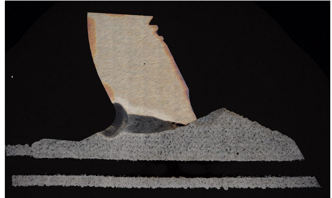
NaOH + NaF etch of Weld 4
